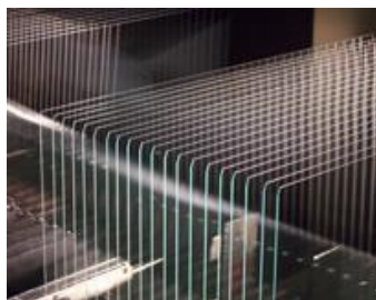
Figure 2.1: Glass substrates coated with a conductive layer of indium tin oxide (9).
