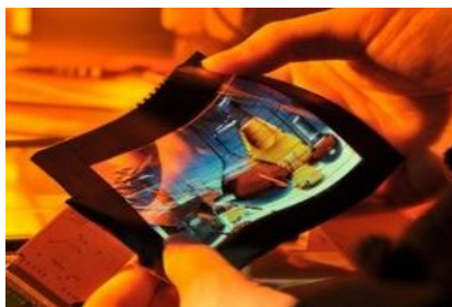
Figure 2.2: Organic light-emitting diode (OLED) display based on mixed oxide TFTs developed by Arizona State University (20).
