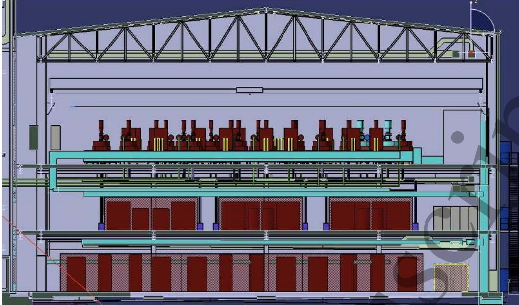
Figure 7. Vertical view of the ITER RF building. The main power supplies are placed on the L1 Ground Level). On level L2, the body and anode (for the JA gyrotrons) power supplies are located. On L3, the gyrotrons and their ancillary facilities, such as superconducting magnets (SCMs), are installed.
