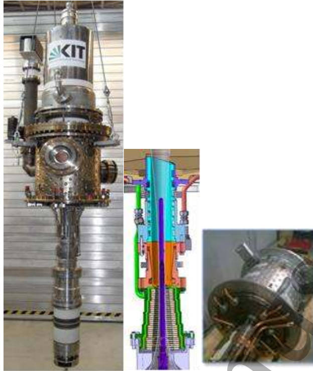
Figure 35. Photo of the upgraded KIT 170 GHz, 2 MW coaxial-cavity pre-prototype to operate at pulse lengths up to 100 ms (left). Sketch of the key components which have been upgraded with advanced cooling systems (middle). Upgrade of the mirror box showing the cooling system (right).
