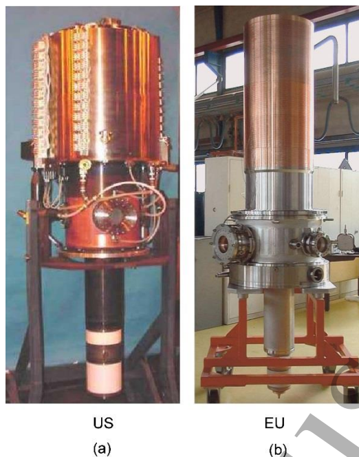
Figure 23. The 140-GHz gyrotrons for W7-X [19] developed by (a) the US (CPI) and (b) the EU team.
