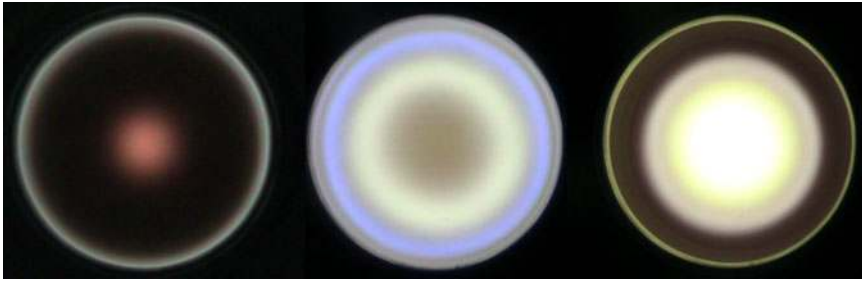
Figure 9. Capacitive (left), low inductive (centre), and high inductive (right) discharge cross-sections for O_2 (30) .
