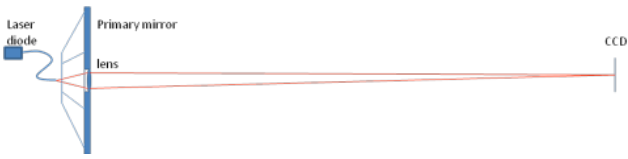
Fig. 9 Laser metrology of the telescope axis tracker. The launcher embedded in the primary mirror substrate forms a 600\ \mu\text{m} (60 pixels) FWHM diffraction limited image of the fiber output on the Telescope Axis Tracker CCD. By sampling the entire 512 \times 512 pixel detector, the parabola axis can be tracked over a 26 arcsec range, with a 0.3 mas estimation error at 10 Hz.
