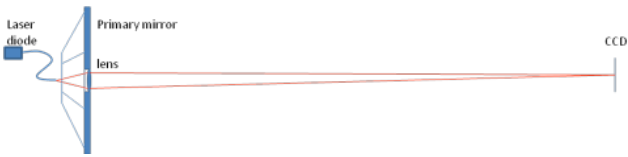
Fig. 9 Laser metrology of the telescope axis tracker. The launcher embedded in the primary mirror substrate forms a 600\ \mu\text{m} (60 pixels) FWHM diffraction limited image of the fiber output on the Telescope Axis Tracker CCD. By sampling the entire 512 \times 512 pixel detector, the parabola axis can be tracked over a 26 arcsec range, with a 0.3 mas estimation error at 10 Hz.
