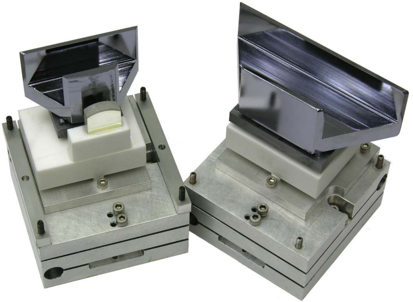
Figure 4. Channel-cut silicon crystals (dark grey) on their aluminum tip-tilt mounts (light grey). The smaller crystal is crystal 1, mounted on the \omega stage. The larger is crystal 2, mounted on the \gamma stage.
