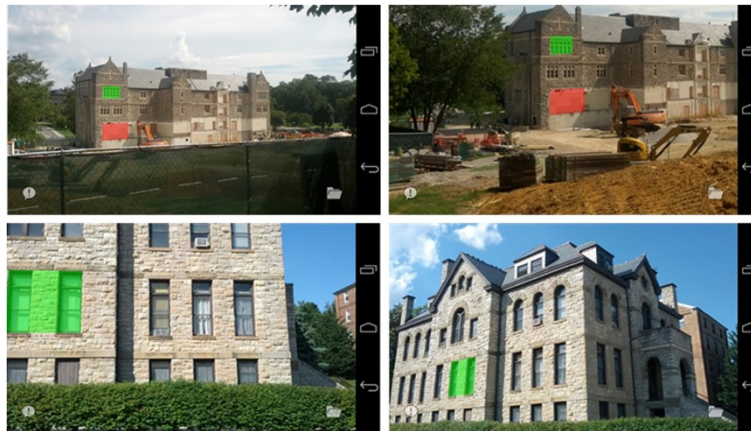
Figure 6 Example of HD 4 AR localization and augmentation. Cyber-information is precisely overlaid on user's photograph despite the significant change of viewpoints.
