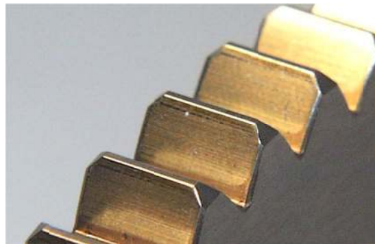
Figure 6.—Photograph of HPA gears after testing.
