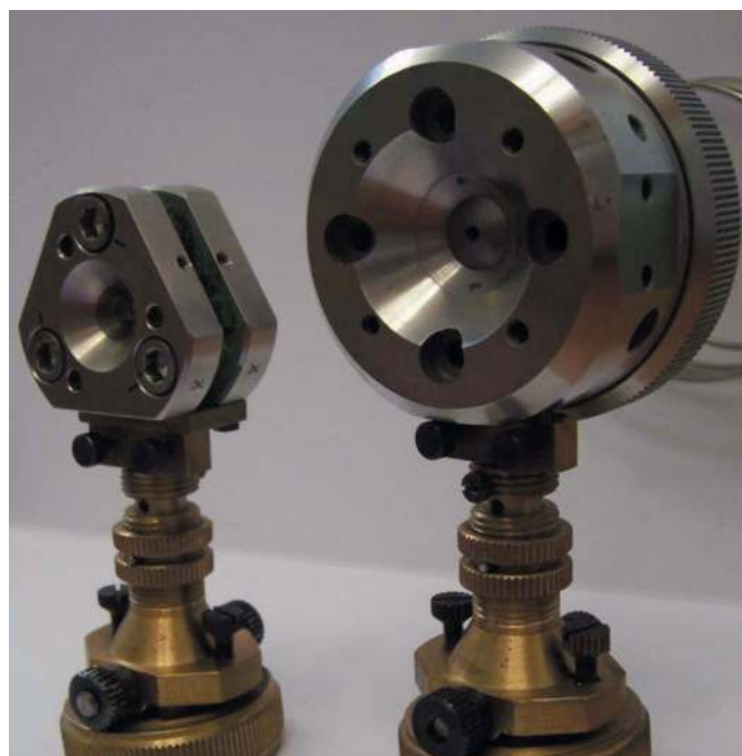
Figure 2 Diamond-anvil cells mounted on goniometer heads: a Merrill-Bassett DAC (Merrill & Bassett, 1974) with steel backing plates of anvils (left) and a gas-membrane DAC with hemispherical beryllium backing plates (right). Behind the membrane cell, the capillary for operating the membrane is visible.
