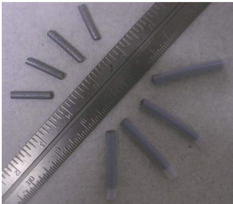
Figure 9: Al / AP / HTPB Strands In and Out of the Teflon Tubing
