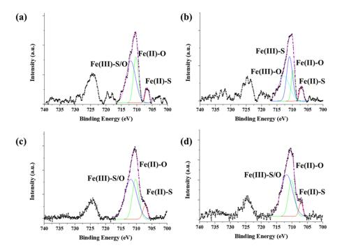
**Figure 8.** XPS spectra of Fe 2p of thermally decomposed catalyst precursors with sulfur: (**a**) ferrocene, (**b**) acetylferrocene, (**c**) ferrocenemethanol, and (**d**) 1,1'-diacetylferrocene.
