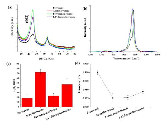
**Figure 2.** (a) X-ray diffraction patterns, (b) Raman spectra of CNTs synthesized with different catalyst precursors, (c)  $I_G/I_D$  ratio, and (d) G mode.
