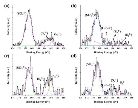
**Figure 4.** XPS spectra of S 2p on CNT bundle: (**a**) ferrocene, (**b**) acetylferrocene, (**c**) ferrocenemethanol, and (**d**) 1,1'-diacetylferrocene.
