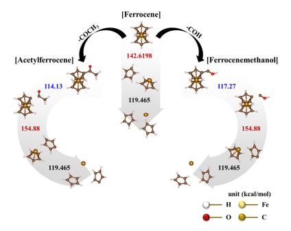
**Figure 6.** Dissociation mechanisms of catalyst precursors based on thermodynamic bond dissociation energy (BDE): ferrocene, acetylferrocene, and ferrocenemethanol.
