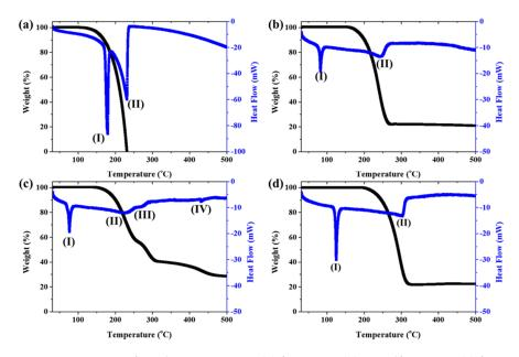
**Figure 5.** TG-DSC of catalyst precursors: (**a**) ferrocene, (**b**) acetylferrocene, (**c**) ferrocenemethanol, and (**d**) 1,1'-diacetylferrocene.
