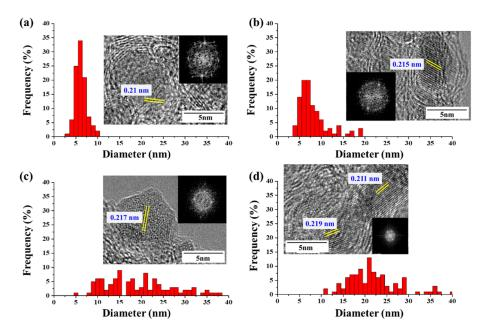
**Figure 3.** TEM images and size distribution of catalyst particles at CNT bundles with different catalyst precursors: (**a**) ferrocene, (**b**) acetylferrocene, (**c**) ferrocenemethanol, and (**d**) 1,1'-diacetylferrocene.
