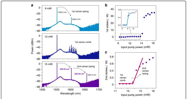
**Fig. 5 Observation of cascaded Raman lasing and threshold measurement. a** First-order Raman lasing at 1603.3 nm with a 204.3 cm<sup>-1</sup> shift from the pump (top). First-order Raman comb generation (middle). Second-order Raman lasing generation (bottom). **b** The first-order SiC Raman laser output power as a function of the input pump power. The inset is a zoom-in of the data in the dotted box. **c** The second-order SiC Raman laser output power as a function of the input pump power
