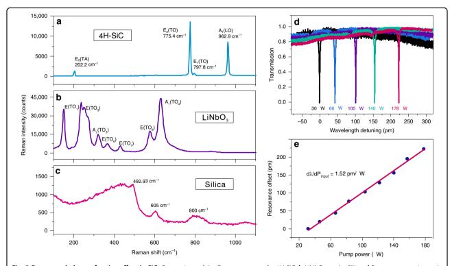
Fig. 3 Raman and photorefractive effect in SiC. Comparison of the Raman spectra of a 4H-SiC, b LiNbO<sub>3</sub>, and c Silica. d Resonance continuously redshifts with increasing of the pump power. e Measured and fitted resonance offset of the microresonator in respect to the pump power.
