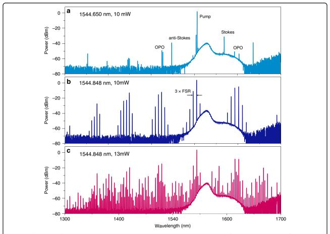
**Fig. 7 Broadband Kerr frequency comb generations in a 4H-SiC microresonator with a radius of 100 um and thickness of 850 nm. a** Measured OPO spectra generated with a launched pump power of 10 mW. **b** Hyper-OPO spectra generation when red-tuned the pump wavelength into resonance near 1544.848 nm. **c** Broadband Kerr frequency comb generations when a 13 mW pump was injected into the microresonator at 1544.848 nm
