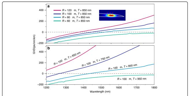
**Fig. 6 Dispersion engineering of the microresonators. a** Dispersion calculation for the fundamental TM mode of the microresonators with a thickness of 850 nm and radius of 60, 80, 100, and 120 μm. Inset show the simulated mode profile of the fundamental TM mode. **b** Dispersion calculation for the fundamental TM mode of the microresonators with a radius of 100 μm and thickness of 650, 750, 850, and 950 μm
