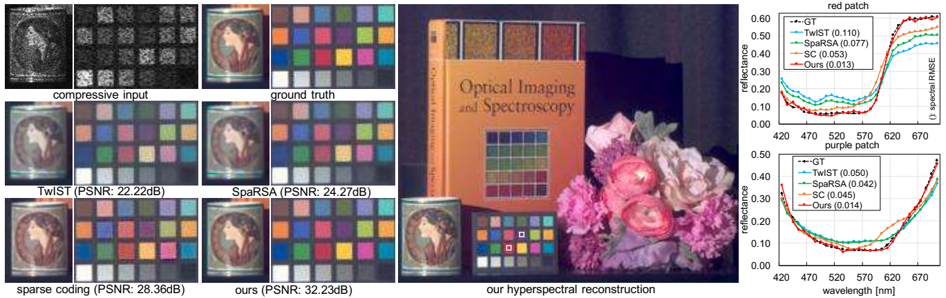
Fig. 1. Our novel hyperspectral reconstruction algorithm works with input from any existing compressive imaging architecture, and yields high-quality results, both in terms of spectral accuracy and spatial resolution. As the comparisons show, our results improve significantly over previous state-of-art methods. For instance, both TwIST and SpaRSA provide suboptimal spatial reconstruction in general, while sparse coding yields a noisy reconstruction of the color chart, and fails to accurately reconstruct the green border in the coffee mug. The charts on the right show how our reconstruction provides an excellent fit to the ground-truth data. In addition, we provide in this work a new high-resolution hyperspectral image dataset.
