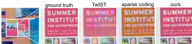
Fig. 17. Limitation example: out-of-focus blur in the input images leads to suboptimal reconstruction of fine details. Nevertheless, our result produces better results than existing approaches.
