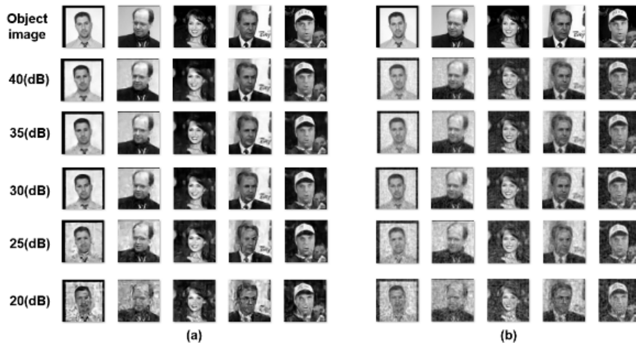
FIGURE 11. Qualitative analysis and comparison of robustness on different levels of detection noises using different models at the sampling ratio of 50%: (a) LR + CGAN model; (b) LR model.
