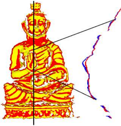
Figure 5. Individual reconstructions are non-rigidly related to each other. The two registered reconstructions are shown in different colours. A zoomed-in cross-section also illustrates the non-rigid deformations present. Please view this figure in colour.
