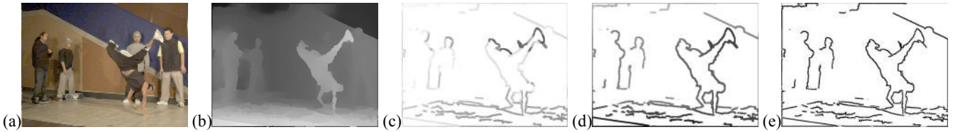
Figure 8: Sample results from matting stage: (a) main color estimates; (b) main depth estimates; (c) boundary color estimates; (d) boundary depth estimates; (e) boundary alpha (opacity) estimates. For ease of printing, the boundary images are negated, so that transparent/empty pixels show up as white.
