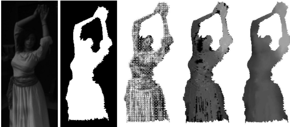
Fig. 8. A 320 \times 240 image taken from a single camera in a stereo cluster (left), a background subtracted image generated for that image (second from the left), the mesh generated for this image (middle), the pre-processed disparity image (second from the right), and the post-processed disparity image (right). Note that lighter gray values indicate that the object in the scene is closer, darker gray indicate that an object in the scene is further away, and black indicates areas of uncertainty.
