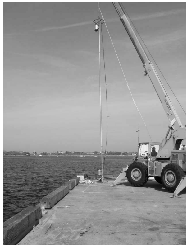
Fig. 3. Both transducers are attached to a 10 m pole.
