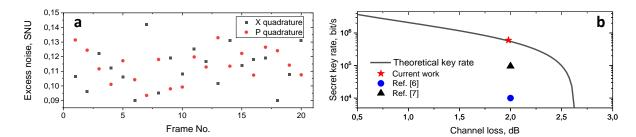
Fig. 2. Experimental results demonstrating our CV-MDI-QKD system performance. (a) Excess noise variance (in shot-noise units). (b) Experimental key rates and numerical simulations.
