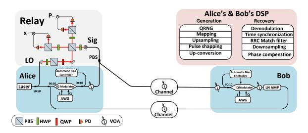
Fig. 1. CV-MDI-QKD system experimental setup and DPS pipeline. AWG: arbitrary waveform generator; PBS: polarization beam splitter; HWP: Half-wave plate; QWP: quarter-wave plate; PD: photodiode; VOA: variable optical attenuator.
