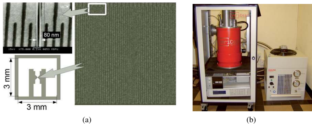
Figure 2. (a) Detector contact pad design and SEM image of the superconducting meander covering a 10\ \mu\text{m} \times 10\ \text{m} area. The strip widths are generally 100–120 nm with spacings of 80–100 nm, respectively. (b) Closed cycle pulse tube cryostat.
