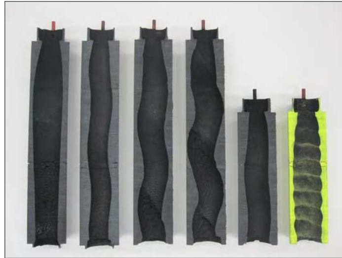
Fig. 4.8: Post-Test Fuel Grain Cross Sections
