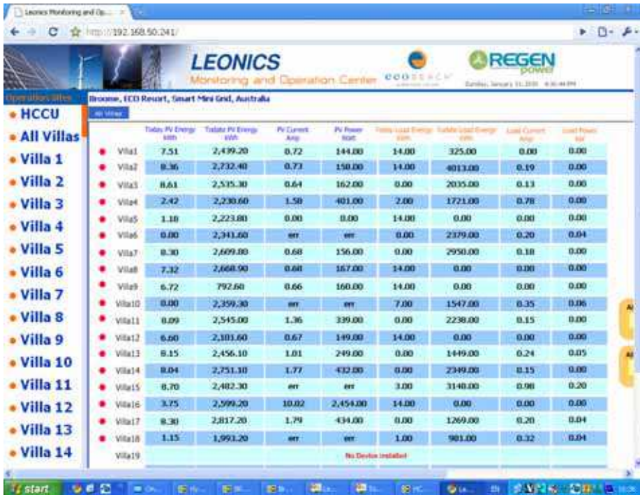
Fig. 23. Monitoring of energy generation and consumption in villas
