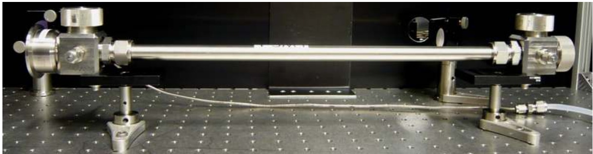
Fig. 8-1 High gas pressure cell for spectral broadening via self phase modulation of the laser beam.
