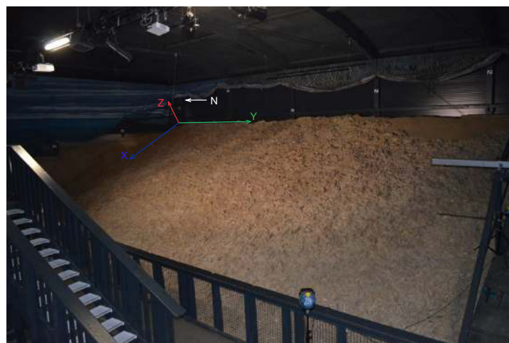
Figure 4. The local analysis coordinate system (LACS) adjusted to the oyster field. Note that the origin is shifted even farther to the back than shown in this figure.
