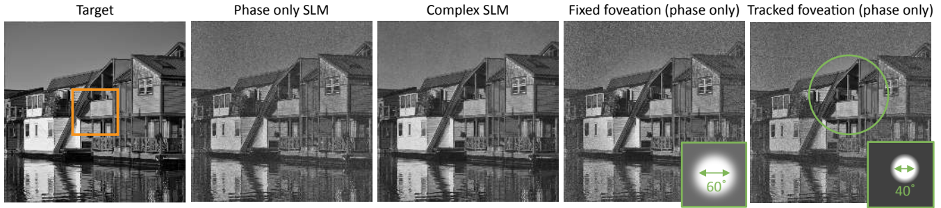
Fig. 8. We propose three methods to further improve contrast for 16\times étendue enhancement beyond the performance of our baseline frequency constrained method (shown in second panel). First, with emerging complex-valued SLM technology, image contrast can be improved over the whole FoV. Second, since the eye tends to rotate only within a limited range before the head moves, in a 120^\circ display a large portion of the FoV is almost always in the periphery. Therefore, we can improve contrast in the center by applying our spatial constraints in a fixed foveation pattern that does not require eye tracking. Finally, if eye tracking is available, our spatial constraints can be used to improve quality in a dynamically changing subregion, highlighted by the green circle. The orange box indicates the native FoV, and the spatial maps used in the foveated simulations are shown in the insets. Floating houses source image by Madeleine Deaton (CC BY 2.0).
