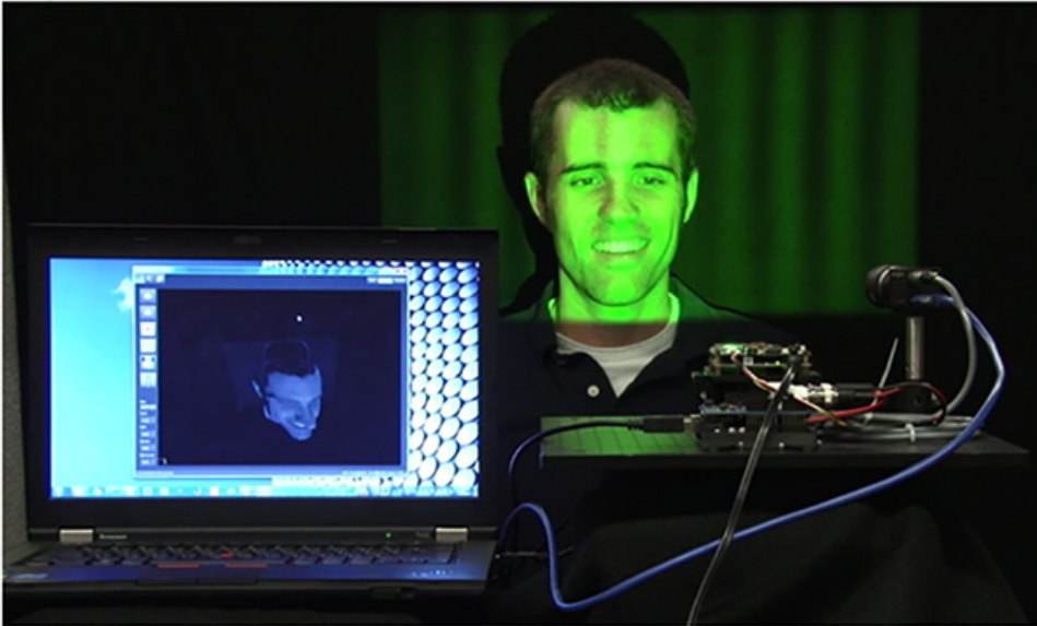
Figure 4. Live 3D video capturing, processing, and rendering. The 3D measurements are displayed in real time on the computer screen to the subject's right.
