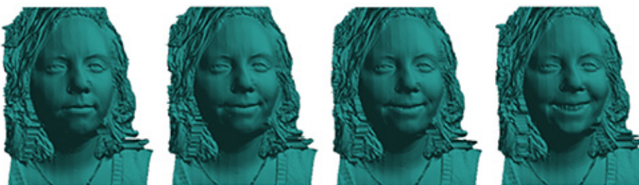
Figure 3. Four selected frames from 3D video of the formation of a facial expression. The video was captured at 60 Hz with a resolution of 640 x 480. These frames highlight the geometric changes in the woman's face as she moves from a neutral expression to a smile.
