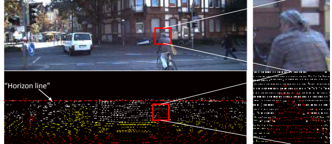
Fig. 1. Example of an urban scene where the LIDAR point-cloud is shown in pixel coordinates (bottom). The sparseness of the LIDAR is emphasized in the zoom view at the bottom-right. This frame is part of the KITTI-dataset, where the LIDAR is mounted on the roof of a vehicle and the LIDAR covers a field-of-view (FOV) limited by a vertical angle - approximated by a line (red dashed). This line will be hereafter called horizon line.
