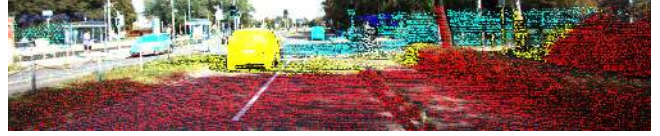
Fig. 4. An example of groundtruth point cloud, superimposed on a color image, with some objects (vehicles) having better resolution than the majority regions in the groundtruth. Those well delineated vehicles, that represent foreground objects, are a challenging situation for a solution using single LIDAR-based point cloud.
