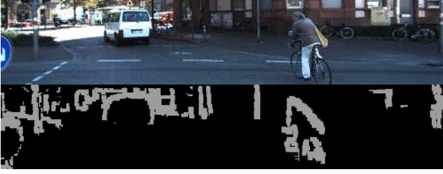
Fig. 3. The first row is an example-frame from the KITTI dataset and serves for visualization purpose; in the row below, the pixels in light-grey indicate the center of masks where nc > 1 hence, corresponding to discontinuities/edges between foreground and background.
