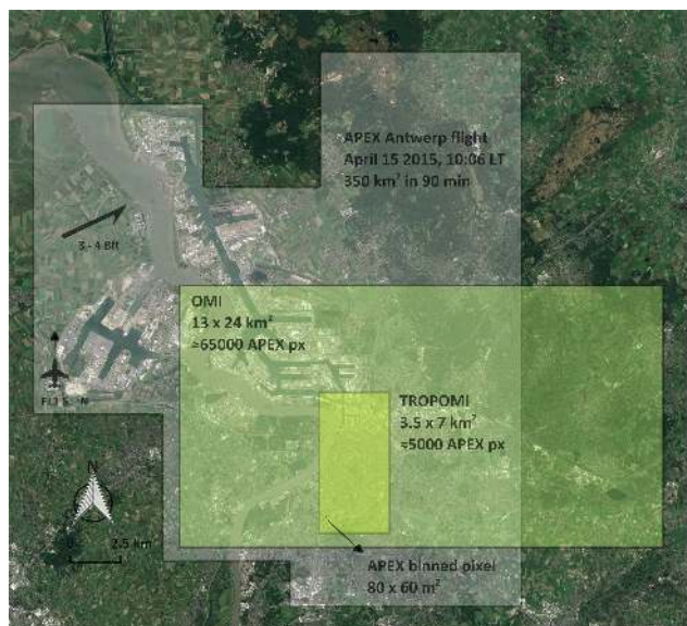
Figure 2. Details of the APEX flight plan over Antwerp on 15 April 2015 and comparison with a space-borne nadir OMI and TROPOMI pixel (Google, DigitalGlobe).
