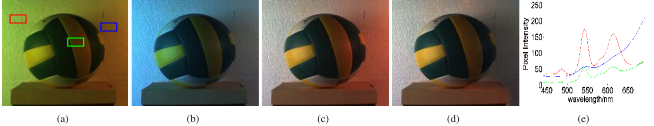
Figure 9. White balance with hybrid illumination. (a) Raw frame captured by the RGB camera. (b) Global white balancing based on fluorescent light. (c) Global white balancing based on tungsten light. (d) Spatially-variant white balancing with our system. (e) Multispectral curves of points with different light blending.
