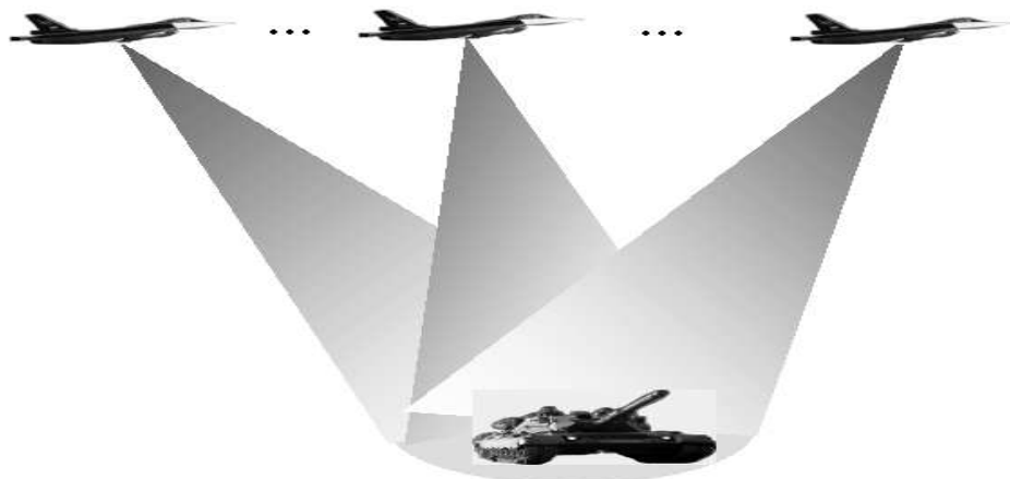
Figure 4.13. SAR imaging with angular diversity.
