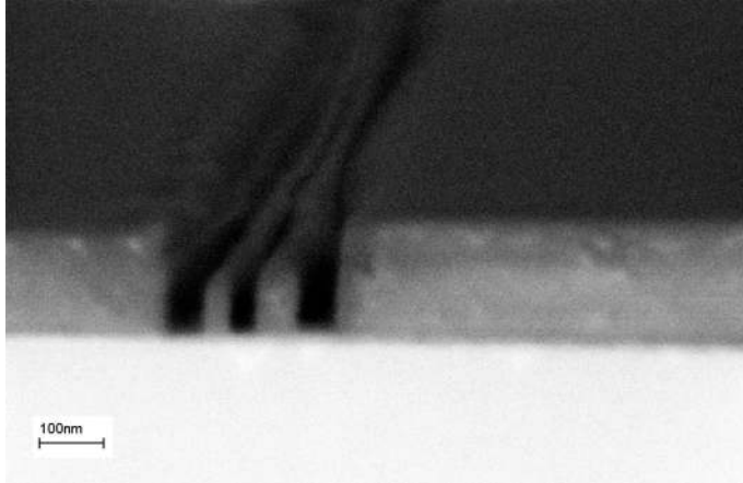
Figure 4.13: SEM image of thermal nanoimprint in PMMA (38 kDa) using the triple Si ridge template as shown in Figure 4.9.
