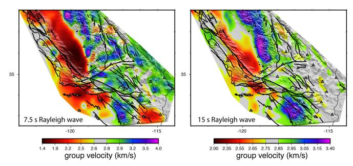
Group speed maps constructed by cross-correlating 30 days of ambient noise between USArray stations in California. Black solid lines show known active faults. White triangles show the locations of USArray stations used in this study.
