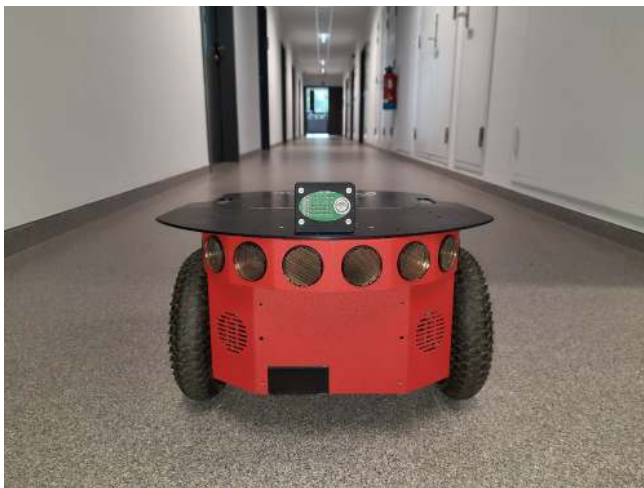
FIGURE 8. Setup of the real-life imaging run of the \mu RTIS. The \mu RTIS is attached to a Pioneer 3-DX and was driven through a narrow corridor of approximately two meters wide at our university.
