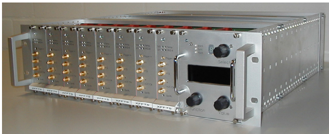
Fig. 5. Photograph of the 19-inch XFFTS-crate, equipped with eight XFFTS-boards (hence processing 20 GHz signal bandwidth) and one FFFTS-controller unit. The modular concept allows combining multiple crates to build large FFT spectrometer arrays.
