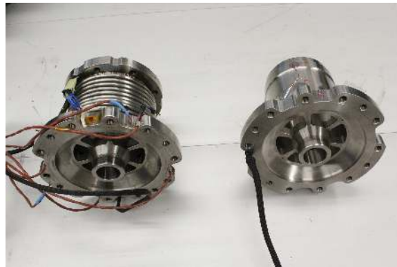
Figure 20. Convoluted Bellows (left) and High-Pressure Air Adapter Coupling (right)
