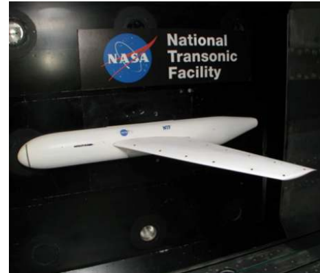
Figure 1. Fundamental Aerodynamic Subsonic/Transonic-Modular Active Control (FAST-MAC) Semi-Span Test at NTF (NASA Langley Research Center)
