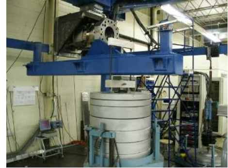
Figure 6. 5.2% NTF-117S Balance Calibration Setup
