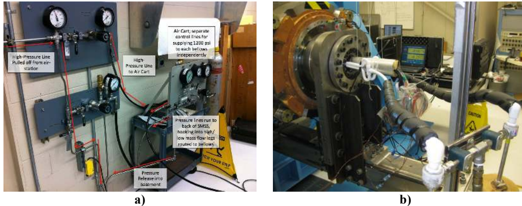
Figure 17. Model Preparation Area, a) Air Cart Configuration, b) Vortex Cooler Configuration
