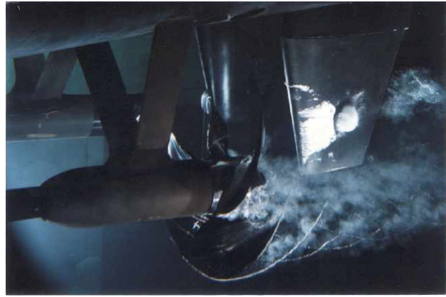
Figure 9. Cavitation visualization of the interaction between a propeller wake and rudder. The propeller diameter is 40.6 cm and the rudder chord at its tip is 18.6 cm. (Photograph: courtesy of Dr Young Shen of NSWCCD.)
