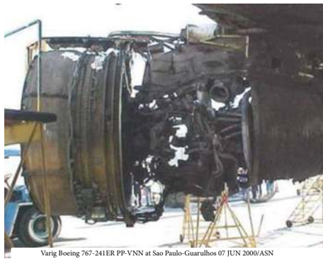
FIGURE 2: CF6-80 engine: fatigue destruction of III-IX stages of HP compressor [24].
