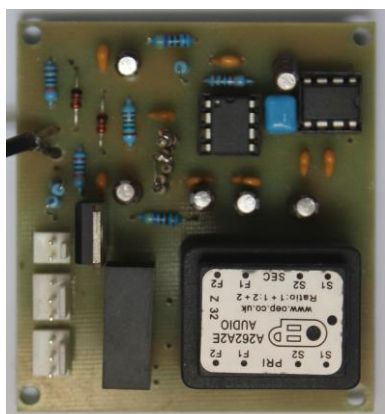
Figure 4. Picture of Realized VLF Receiver Deployed on a PCB
