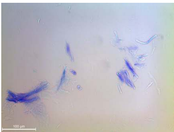
Fig. 1 TEMPO-oxidised CMF/CNF under optical microscope at \times 500 magnification
