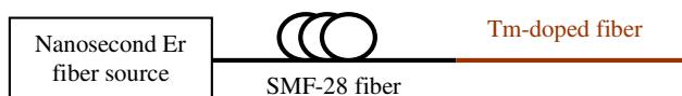
Fig. 1. (Color online) The experimental setup. SMF-28 fiber: \sim 5 m. Tm-doped fiber: \sim 50 cm.
