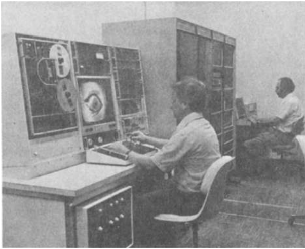
Figure 4. The operator's console and the data-reduction facility. The CRT and hard-copy printer can be seen on the far right.
