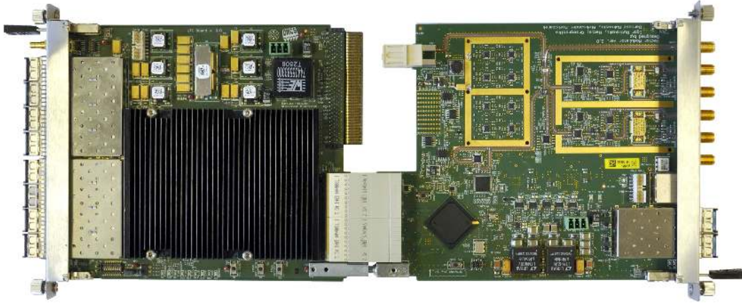
Fig. 3. The photograph of the DAMC-TCK7 data processing module (on the left) connected with a Vector Modulator (on the right)
