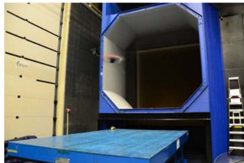
Fig. 1. Figure of Open Jet Facility and the spinning quadrotor during flight.
