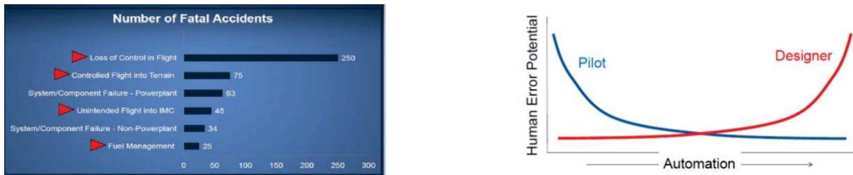
Figure 12 : NTSB Compiled Data for Personal Aviation Indicating the Cause of Accidents (left) and the Relationship of Human Error Potential Induced by the Pilot or Automation Designer
