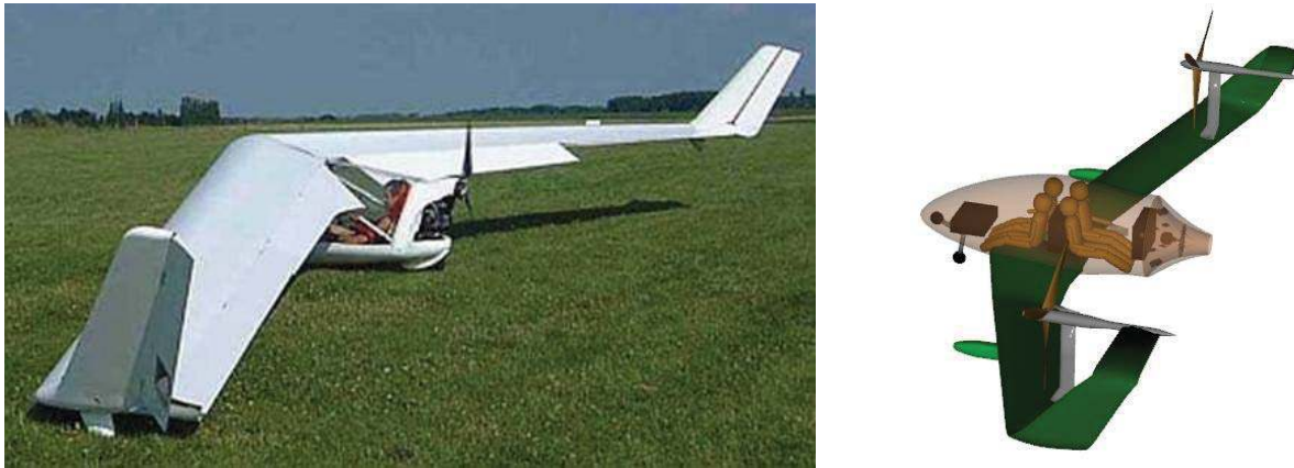
Figure 16: SWIFT Single Person Sailplane (left) and Zip e-SWIFT Concept (right) for Moderate Speed/High Aerodynamic Efficiency
