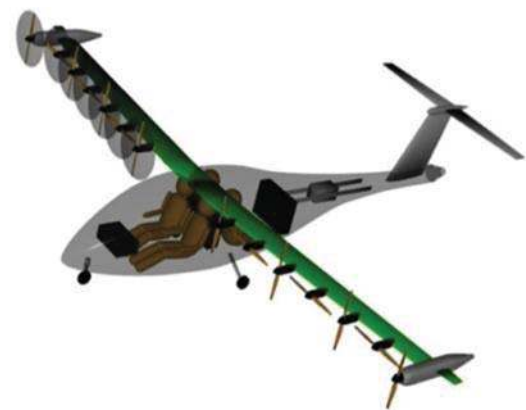
Figure 17: Zip e-ATLIT High Speed, High Wing Loading, Highly Distributed Concept
