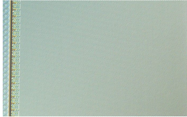
Figure 10: DIC microscopy image of pixel area after sacrificial layer etch. Minimal and homogeneous tilt of idle mirrors.
