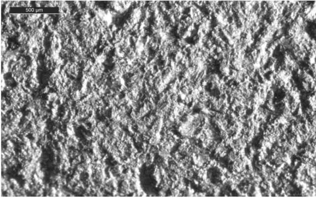
Figure 10. Wear surface of an AISI 316 sample.
