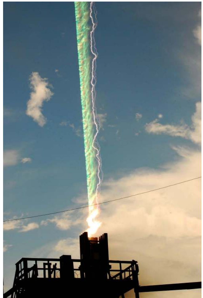
Figure 3. Photograph of the first rocket triggered lightning flash described in this report, recorded on 15 July 2010. The exploded triggering wire is on the left, the wind-separated dart leader-return stroke channel on the right. The rocket-launch tubes, also visible on top of the tower in Figure 1, can be seen at the bottom of the picture (courtesy of D. Hill).
