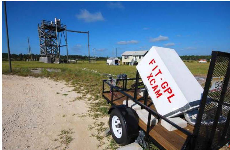
Figure 1. Photograph of the X-ray camera in front of the rocket-launch tower used to trigger lightning at the ICLRT (courtesy of D. Hill).
