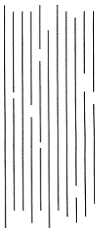
Figure 1. Ideal polymer chains model for producing high strength and high modulus fibers.
