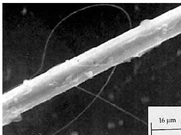
Figure 15. A single electrospun PPTA fiber together with a single Kevlar ® 49 fiber [100]. Reproduced with permission from Srinivasan & Reneker, 1995. Copyright John Wiley & Sons.
