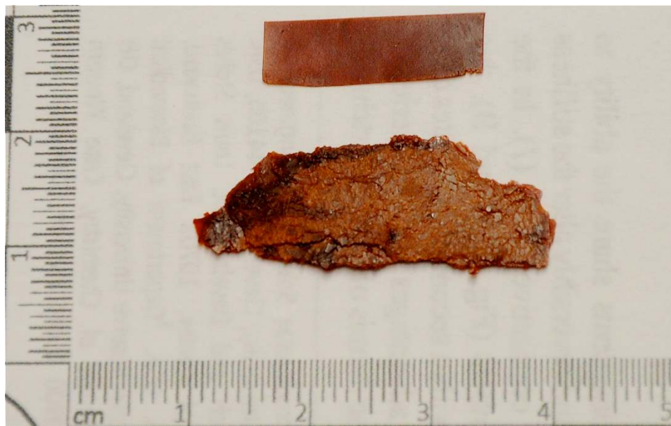
Figure S5. Image of 20 wt.% nanocomposite films as cast from solution (top sample) and after melt processing at 85 °C and 200 kPa (bottom sample).
