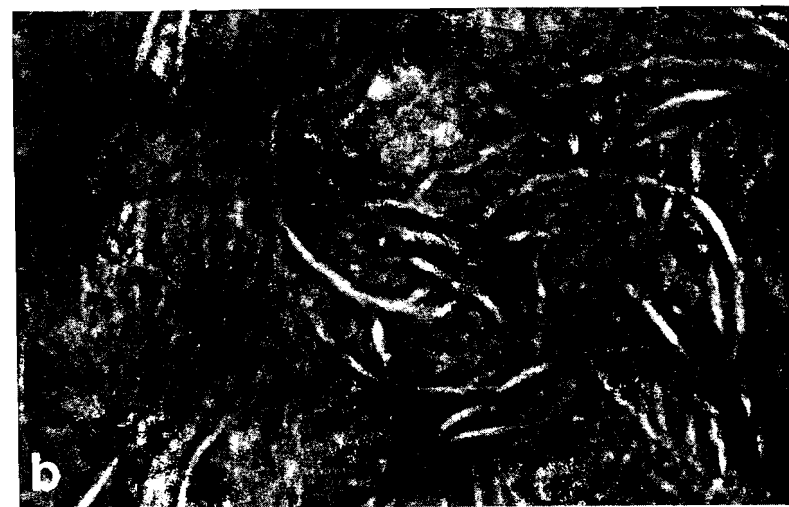
FIG. 14. Morphology of (a) solution-crystallized (cast from 1.5% solution in decalin) UHMW-PE and (b) recrystallized sample (heated to 150°C for 60 s and quenched).
